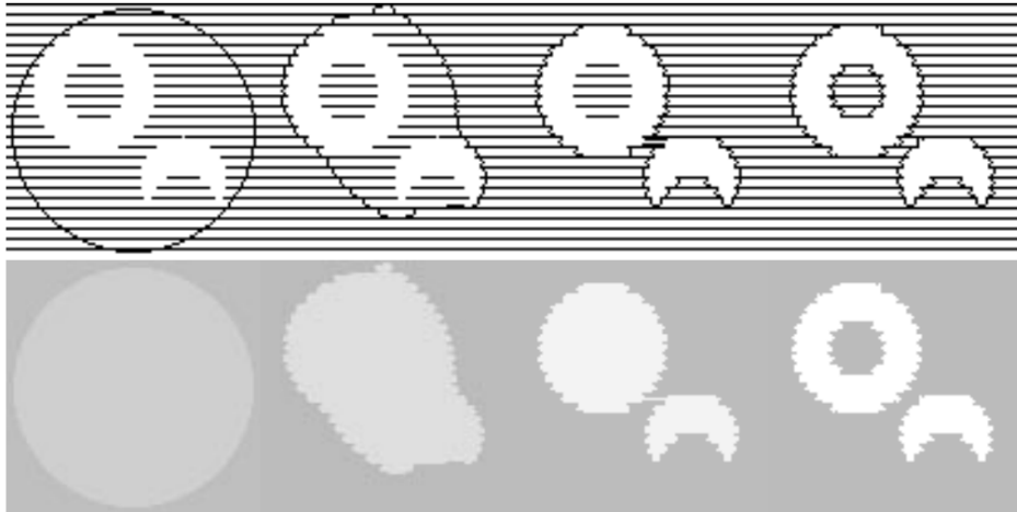
Figure 3: This is to illustrate the fact that the model can detect boundaries without using the gradient. The top row represents evolving contour and the bottom row represents piecewise constant approximations: c_0 and c_1
